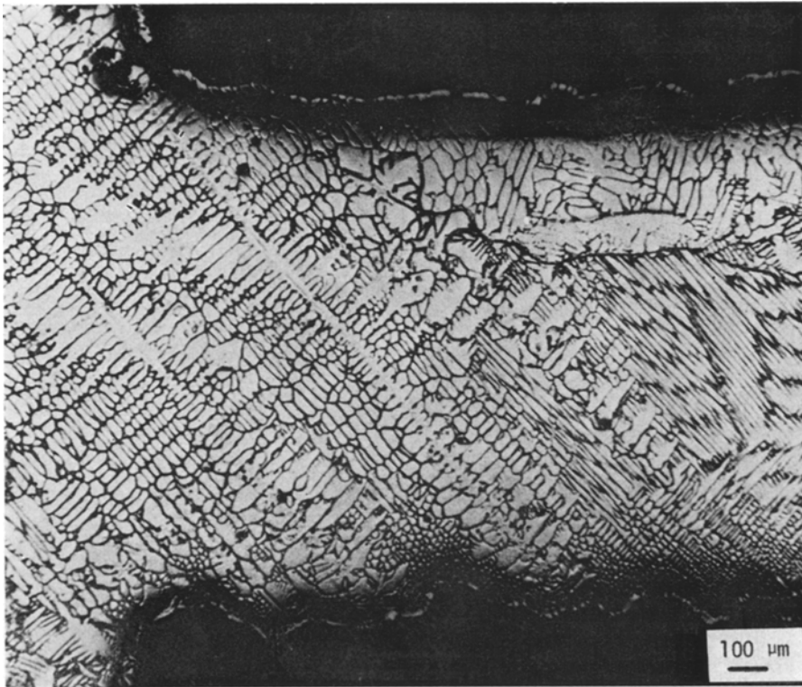
Figure 5 Cross-section of as-cast lead acid storage battery grid, Pb-0.075 wt % Ca-1.0 wt % Sn alloy. (Courtesy of T. W. Caldwell, NL Industries.)
